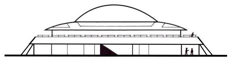
Building of 44 m outside diameter; inside dome diameter of 20 m (120 seating) with 2.5 m edge height. Offices, museum and exhibition space 6 m deep on first floor, 11 m deep on ground floor; total usable space around the dome cylinder of 1500 m<sup>2</sup>. Dome cylinder 315 m<sup>2</sup>. Building material: all wood with copper sheating.
