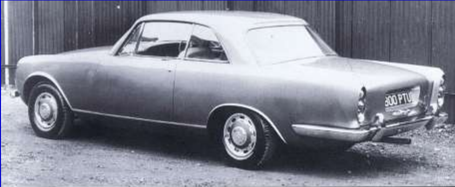
Built on chassis 61-B, this Korea prototype car had a Park Ward body. Note the sleek styling and Bentley wheeltrims. (Courtesy Rolls-Royce Motor Cars Ltd.)
