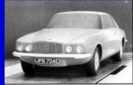
A further styling theme was a proposed Continental version of Burma, known as Korea. The wax model pictured here shows the car's sporting attitude and remarkably modern frontal appearance. (Courtesy Rolls-Royce Motor Cars Ltd.)
